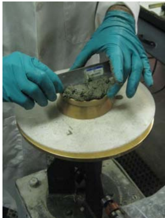
4. Cut off Mortar Plane with Sawing Motion with Straightedge or Trowel.
